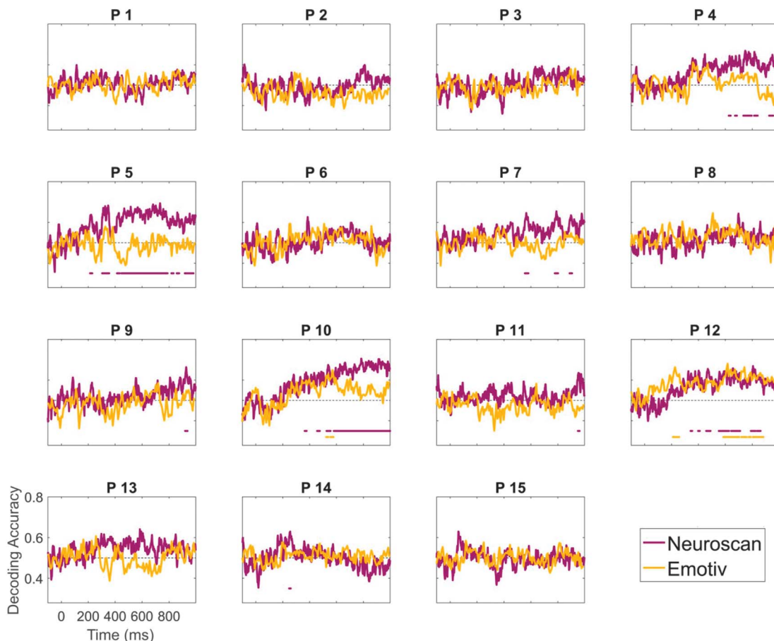
Figure 7. Experiment 1 (word pairs) individual participant decoding accuracy for classification of congruent versus incongruent conditions over time for Neuroscan (purple) and EPOC+ (yellow) data. Time points with accuracy significantly above chance ( p < .05 assessed with threshold-free cluster enhancement permutation tests corrected for multiple comparisons; see Method section) are shown as solid horizontal lines (in purple for Neuroscan and yellow for EPOC+). Theoretical chance (50%) is indicated by the horizontal dashed line. Semantic condition could be decoded in eight of 15 (53%) individuals' Neuroscan data and in two of 15 (13%) individual's EPOC+ data. P = participant.
